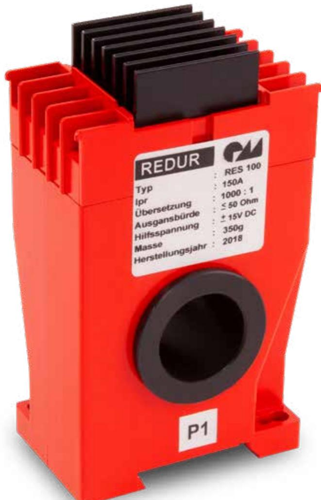
With our RES 100 current transformer, you can measure even the smallest current fluctuation in the grid, because it detects currents from 0 (DC) up to 500 kHz (AC) at 100 ppm accuracy. This superb accuracy is based on the Zero-Flux™ technology that guarantees a high linearity as well as small frequency and phase errors.
