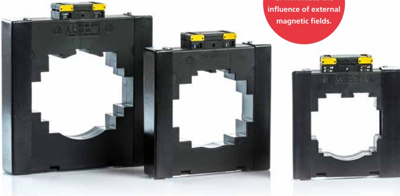
The busbar typ CTs for indoor applications is characterised by its compactness, multifunctionality and high safety requirements. This type of CT minimises the influence of external magnetic fields, which can negatively impact the accuracy of current transformers at high currents and small distances between busbars. All current transformers comply with IEC 61869 (DIN EN 61869/VDE 0414, DIN 42600).
